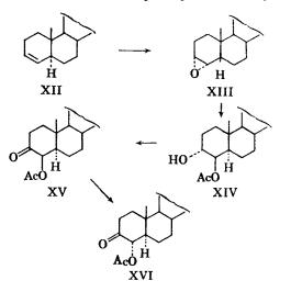
The latter substance was oxidized in 87% yield to  $4\beta$ -acetoxycholestane-3-one (XV), m.p. 133.7-134.4,  $[\alpha]_{\rm b}$  +57°, after purification. Epimerization of this axial acetoxy ketone with hydrobromic acid in acetic acid gave an 89% yield of  $4\alpha$ -acetoxy-cholestane-3-one (XVI), m.p. 144-145°,  $[\alpha]_{\rm b}$  -3.7°, after purification.
